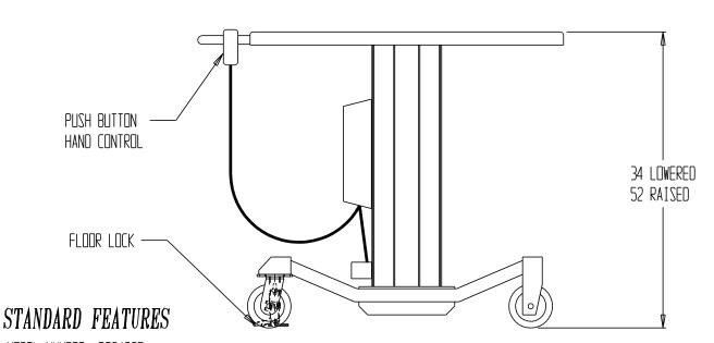
MODEL NUMBER: PT2436E CAPACITY: 1,000 LBS. DECK SIZE: 24"W x 36"L
